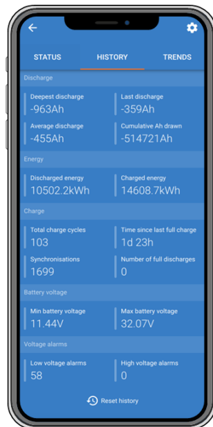
The VictronConnect app battery monitor history screen.
