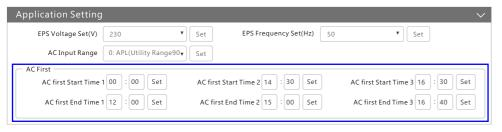
AC First: During the setting time, system will use AC to take load first, use solar power to charge the battery. If the battery is full, solar power may be wasted. When out of the setting time, system will use battery and solar to take load until battery voltage/SOC is lower than cut off voltage/SOC
