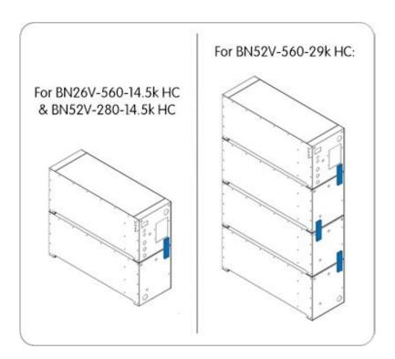
Connect the enclosures in series: B1(-) to B2(+); B2(-) to B3(+); B3(-) to B4(+) etc. as illustrated.
