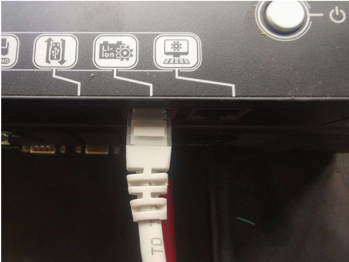
Fig 3.2 Axpert Port for RS485 Cable Coming from the Converter RS485 Output Lead.
