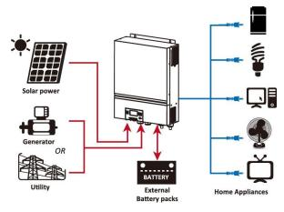
Figure 1 Basic hybrid PV System Overview
