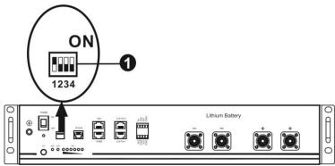
①Dip Switch: There are 4 Dip Switches that sets different baud rate and battery group address. If switch position is turned to the "OFF" position, it means "0". If switch position is turned to the "ON" position, it means "1".
