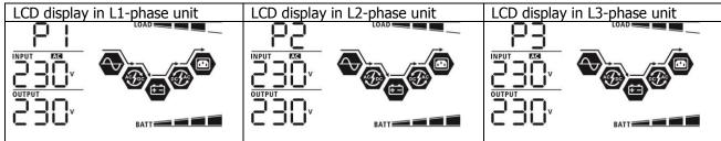
Step 5: If there is no more fault alarm, the system to support 3-phase equipment is completely installed.
