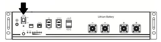
Step 3. Press more than three seconds to start Lithium battery, power output ready.
