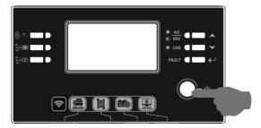
Step 4. Be sure to select battery type as "SOL" in LCD program 5.
