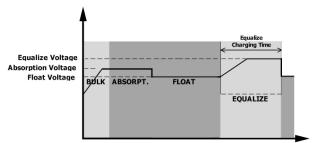
However, in Equalize stage, when battery equalized time is expired and battery voltage doesn't rise to battery equalization voltage point, the charge controller will extend the battery equalized time until battery voltage achieves battery equalization voltage. If battery voltage is still lower than battery equalization voltage when battery equalized timeout setting is over, the charge controller will stop equalization and return to float stage.
