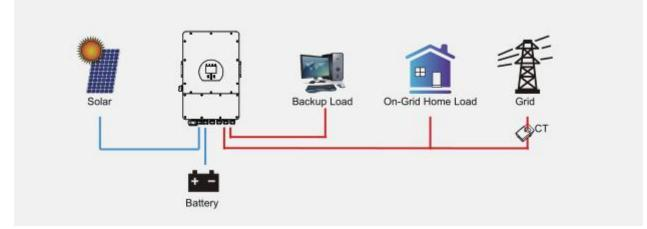
Hybrid inverter will not only provide power to the backup load connected but also give power to the home load connected. If PV power and battery power is insufficient, it will take grid energy as supplement. The hybrid inverter will not sell power to grid. The external CT(&Meter) will detect power flowing back to the grid and will reduce the power of the inverter only to supply the local load, charge battery and home load. This control is achieved by:
