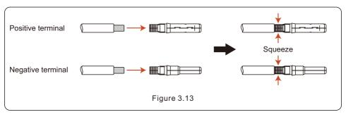
5. Insert the crimped DC cable into the DC terminal firmly, then insert the waterproof rubber ring into the DC terminal and tighten the nut.
