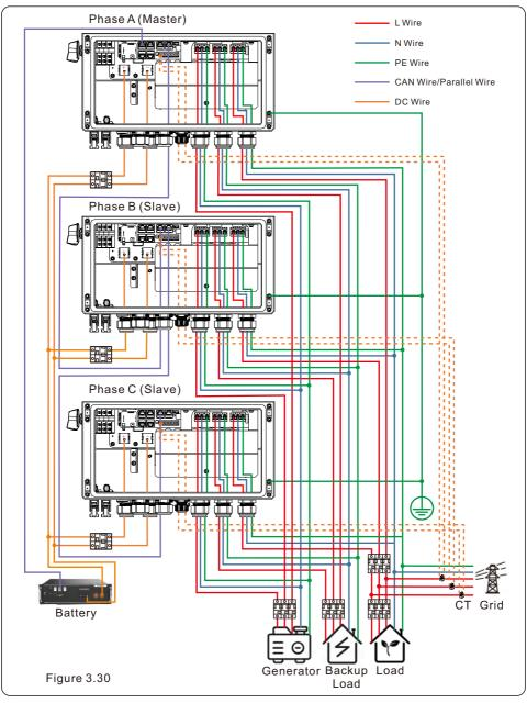
When multiple inverters are connecting in parallel, ONLY same model (same power rating) can be used.
