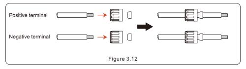
4. Connect the wire part of the DC cable to the metal DC terminal and crimp it with a special DC terminal crimping tool.
