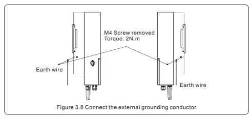
To connect the grounding terminal on the heat sink, please follow the steps below:
