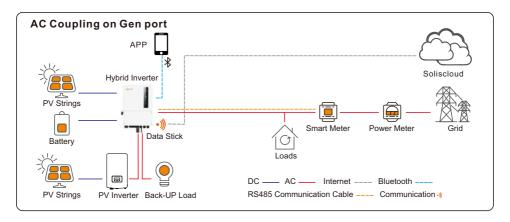
The settings about AC coupling under the smart port setting. When the AC Coupling switch is turned on, customer should set the position is GEN port or Backup port. and set the AC\_Coupling \_OFF\_SOC and AC\_Coupling \_OFF\_VOLT and AC\_Coupling Max.fre. AC\_Coupling \_OFF\_SOC: When the lithium SOC rises to this set value, the grid-tied inverter stops working through load reduction.
