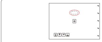
Figure 3.4 Handles used to move the inverter shown circled in red - one per side
