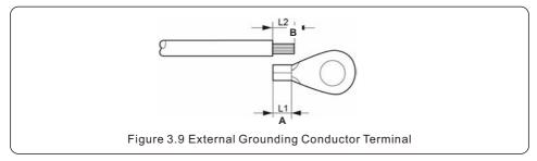
5. The external grounding conductor is recommended to be connected to 4mm2 and above.
