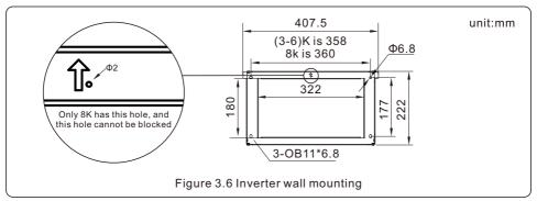
Once a suitable location has be found accordingly to 3.1 using figure 3.6 mount the wall bracket to the wall.
