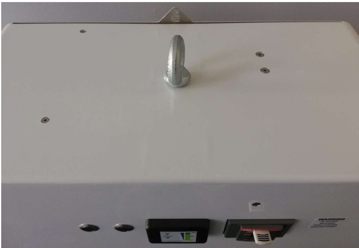
Figure 4.3 Eye bolt Installation on a Lite 15/12HV model (remove after installation)
